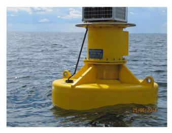
In cooperation with Navigationsteknik, Ocean Origo offers fully equipped data buoys ready for deployment including all necessary components like battery bank, solar panels, nautical equipment, GPS alarm, etc. We also offer complete mooring solutions and mooring components including SeaFlex system for minimizing mechanical mooring stress and customized www-interface. Finally, we also offer installation, service, surveillance and management of buoy systems. In short – we can do it all.
