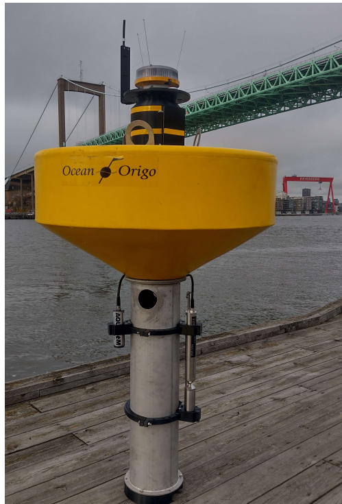
MEMO, here equipped with TRIOS sensors, LoRa communication antenna and X-large batteries.
